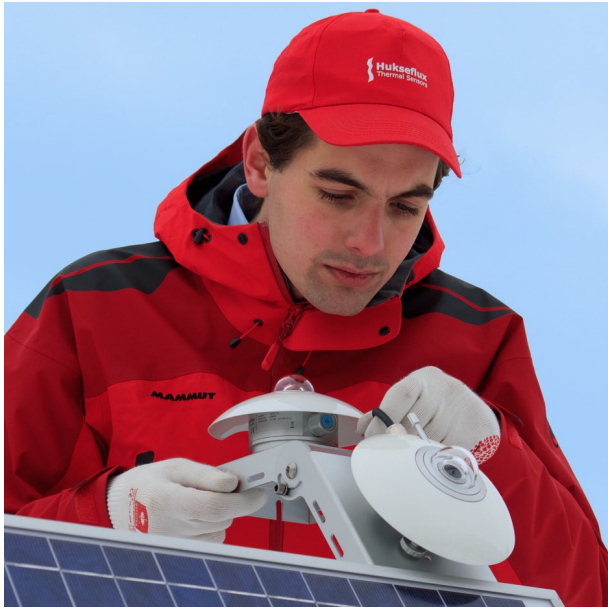
Figure 1 SR20 secondary standard pyranometers in PV system performance monitoring, measuring global and plane of array irradiance
