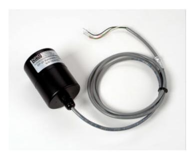
The NRG #BP20 barometric pressure sensor is a micromachined absolute pressure sensor which provides a high level voltage output signal that is proportional to absolute pressure. It includes built-in temperature compensation, linearization, and an output amplifier.
